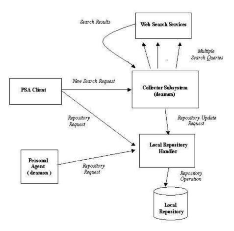
Overall System Architecture of the PSA (Fig I)
